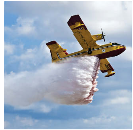
The Super Scooper is a firefighting airplane which can quickly ingest water from a lake by skimming across the surface with just a bottom-mounted scoop entering the water. The mass within the aircraft boundary varies during the scooping operation as well as during the dumping operation shown.
