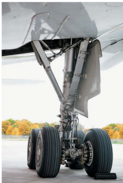
Portions of the landing gear for a large aircraft undergo three-dimensional motion during retraction and deployment.
