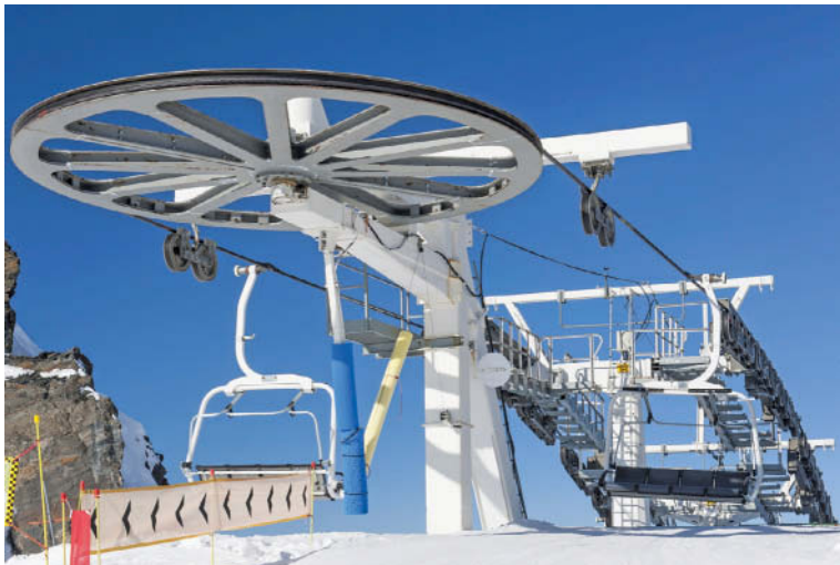
Cable-pulley systems are an integral component in many transportation systems, including this ski-resort chairlift.
