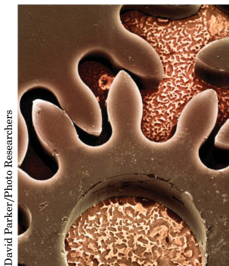
These nickel microgears are only 150 micrometers ( 150(10^{-6}) m) thick and have potential application in micro-robotics.
